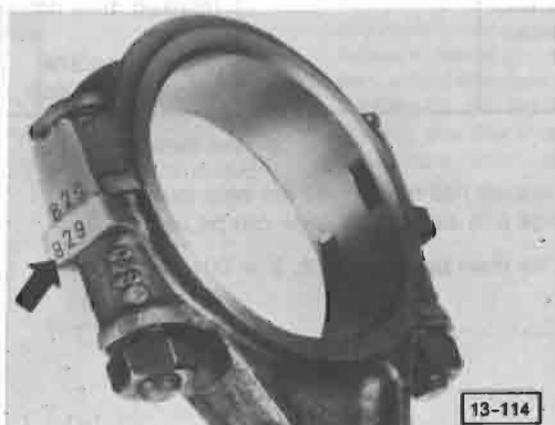
Fig. 6 Connecting rod, installing
