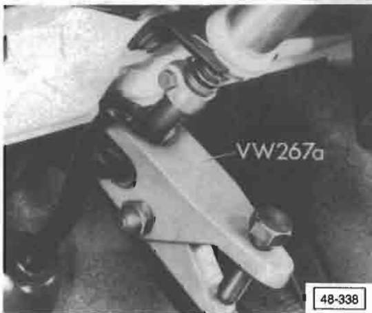
Fig. 2 Steering lock housing/spacer sleeve, installing — when installing spacer sleeve, clamp steering column at top and bottom
