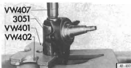
Fig. 8 Lower ball joint, removing
