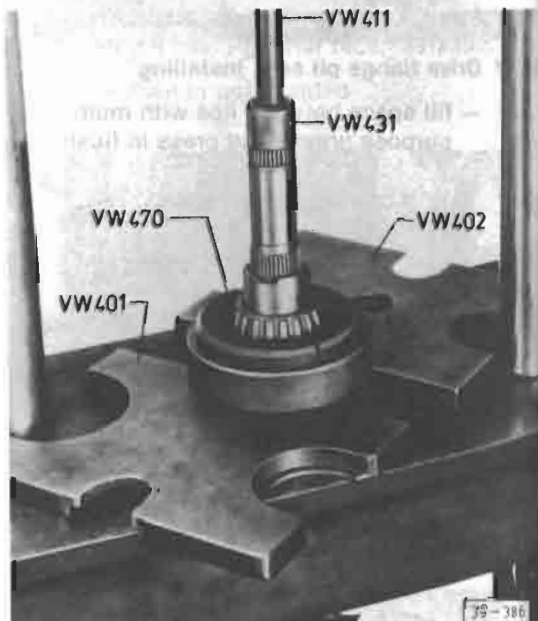
Fig. 18 Pinion bearing inner race/Oil seal sleeve, removing
