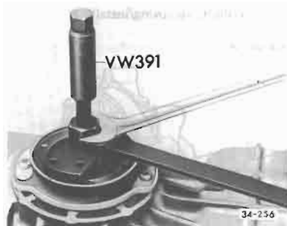
Fig. 7 Drive flange, installing
