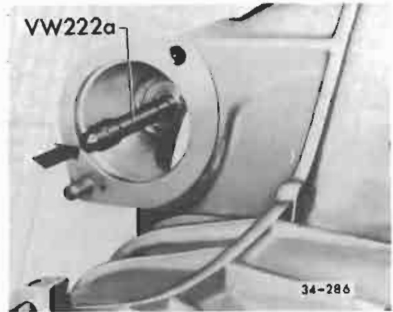
Fig. 4 Starter bushing, installing —lubricate bushing and drive in flush
