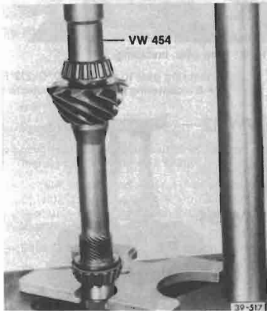
Fig. 20 Pinion bearing inner race, installing
