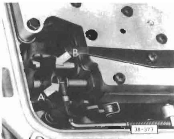
Fig. 1 Valve body, installing
