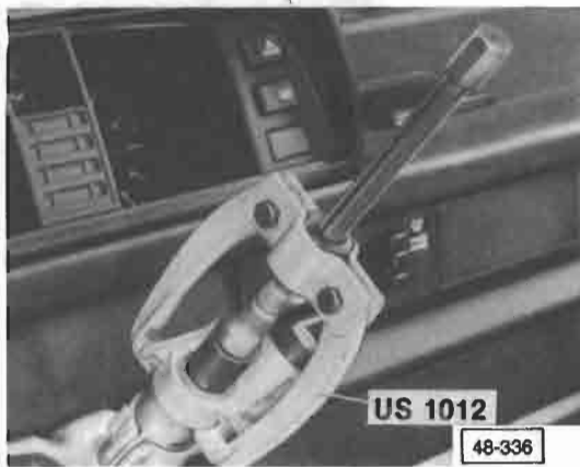
Fig. 1 Steering lock housing, removing — pull off steering lock housing together with spacer sleeve
