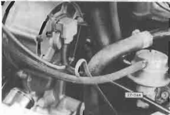
Fig. 2 Voltage regulator, removing and installing
