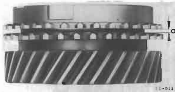
Fig. 2 Synchronizer rings 3rd/4th gears, checking —press synchronizer rings onto gear by hand and measure gap a with feeler gauge
