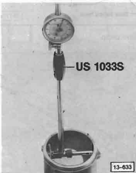
Fig. 11 Cylinder sleeve, checking for wear
