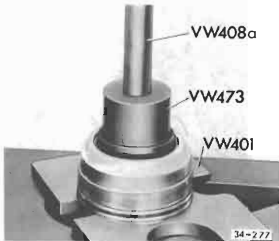
Fig. 1 Drive flange oil seal, removing
