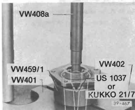
Fig. 16 Pinion bearing outer race in cover, removing
