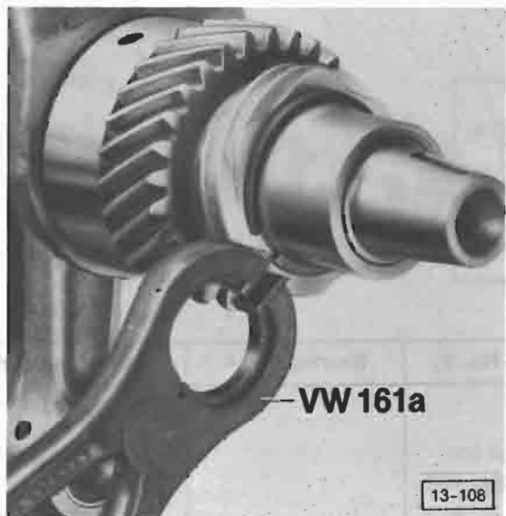
Fig. 2 Circlip, removing
