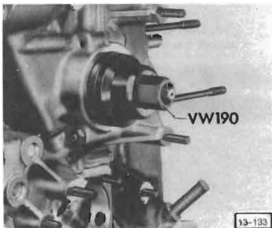
Fig. 7 Crankshaft oil seal, cooling fan side, installing
