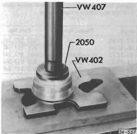
Fig. 11 Differential bearing/outer race, installing — press race in until seated
