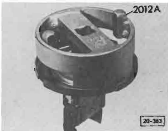
Fig. 3 Fuel gauge sending unit, removing
