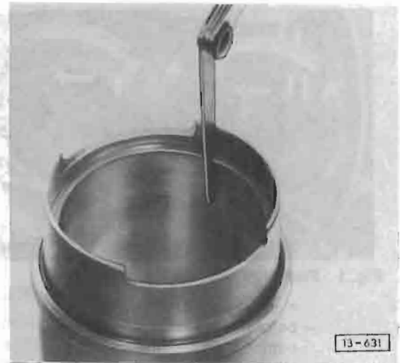
Fig. 8 Piston ring end gap, checking
