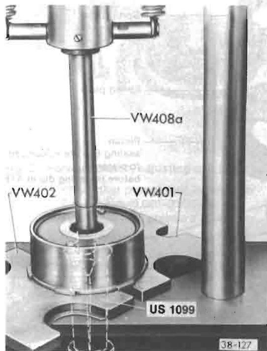
Fig. 2 Bushing in clutch drum, removing — press out
