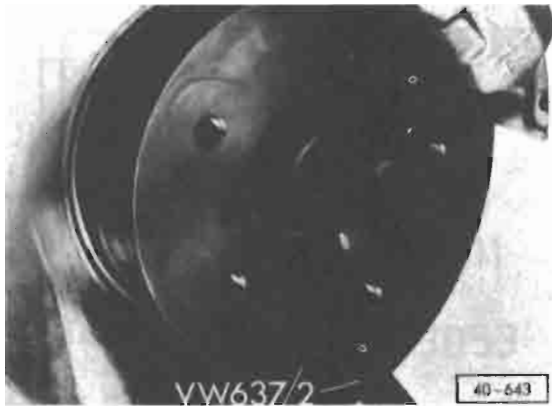
Fig. 1 Grease cap, removing
