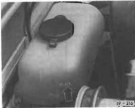
Fig. 4 Cooling system, filling —fill reservoir up to mark max (arrow)
