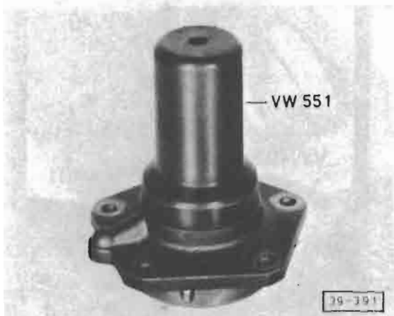
Fig. 15 Pinion oil seal (outer) in cover, installing — drive seal into cover until flush. Open side of seal faces transmission
