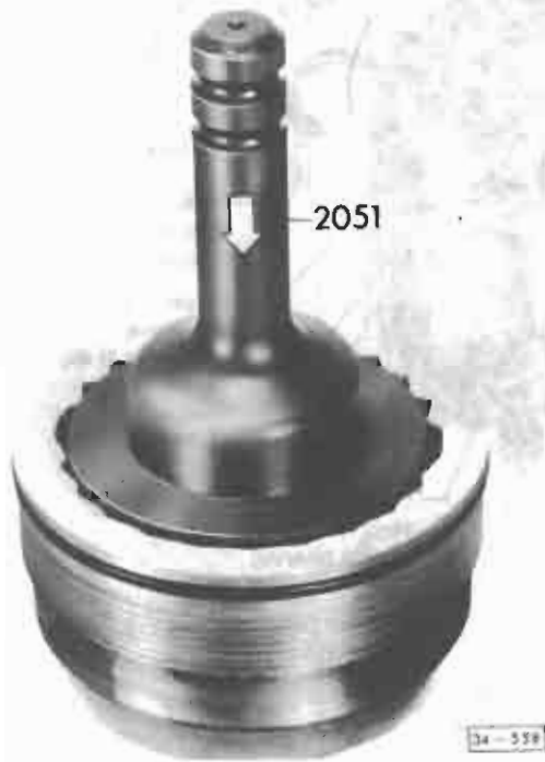
Fig. 2 Drive flange oil seal, installing
