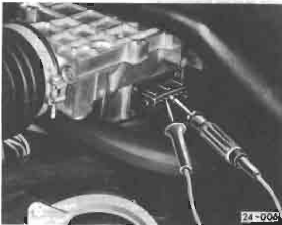
Intake air sensor, checking
