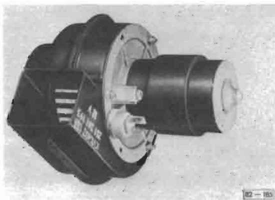
Fig. 20 Air circulation blower, checking (blower installed)
