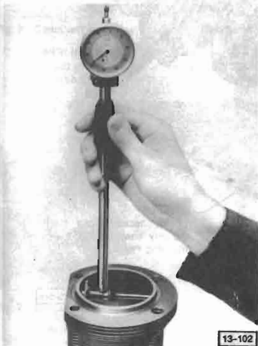
Fig. 9 Cylinder, checking for wear
