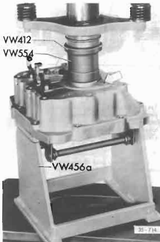
Fig. 11 Main shaft ball bearing, installing
