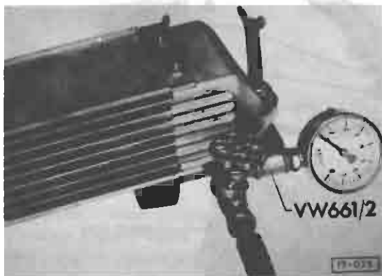
Fig. 3 Oil cooler, checking for leaks
