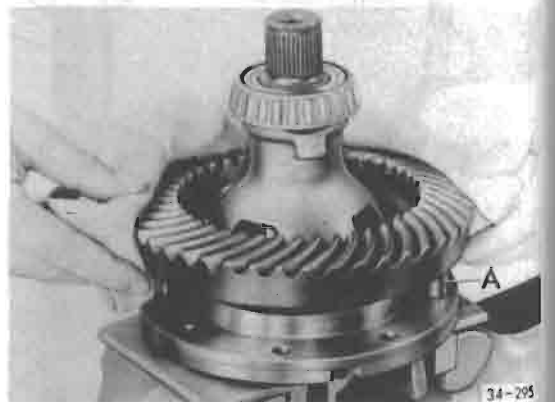
Fig. 9 Ring gear, installing
