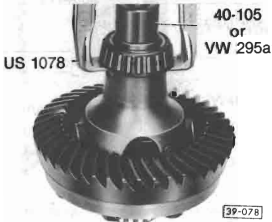
Fig. 1 Differential bearing/Inner race, removing
