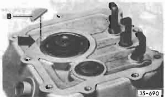
Fig. 4 Main shaft bearing locking key B, installing
