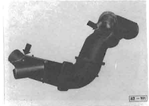
Fig. 25 Control flaps, checking
