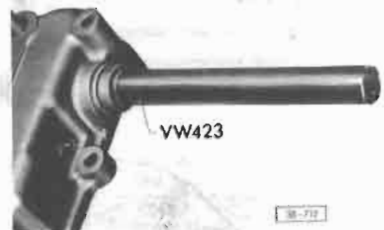
Fig. 6 Selector shaft oil seal, installing — fill space between lips with multi-purpose grease
