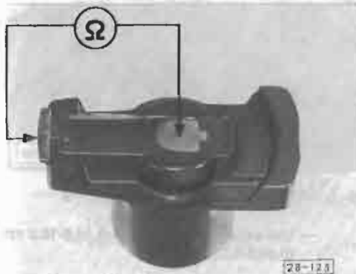
Fig. 1 Rotor, checking
