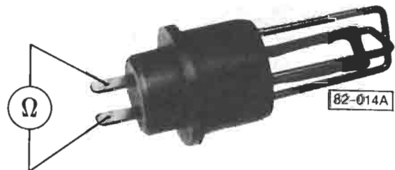
Fig. 13 Temperature sensor, checking
