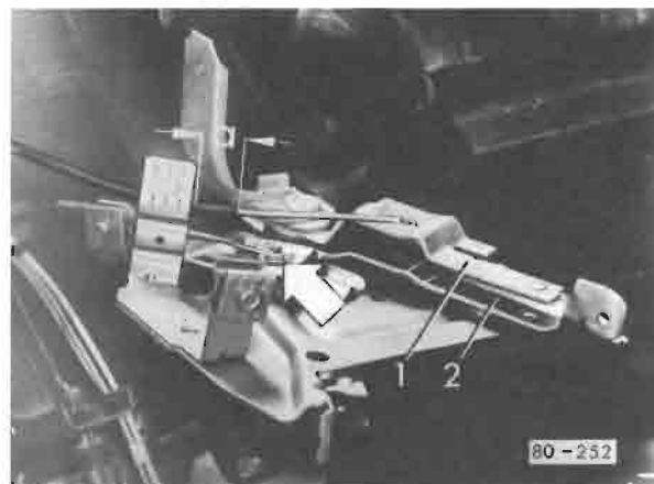
Fig. 3 Control cable on lever 1 -- heated air distributor in passenger compartment cable conduit has red paint mark and projects out of clamp approx. a = max 30 mm ( 1 3/16 in. ) on lever 2 -- heater flap cable (arrow)
