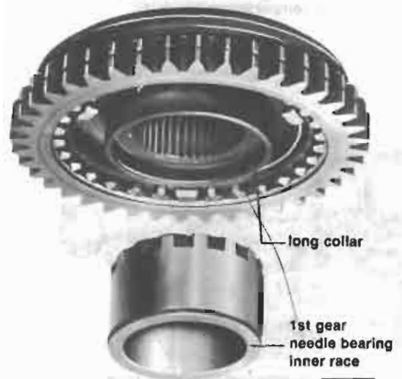
Fig. 12 Synchronizer assembly 1st/2nd gear and 1st gear needle bearing inner race, installation position
