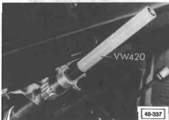
Fig. 3 Steering lock housing/spacer sleeve, installing — note dimension a of Fig. 4
