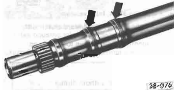
Fig. 5 Turbine shaft rings, checking
