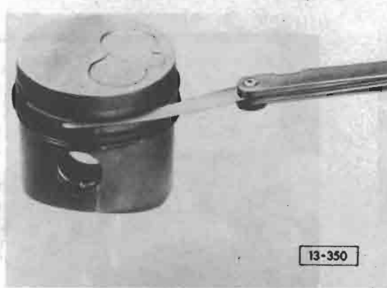
Fig. 7 Piston ring side clearance, checking
