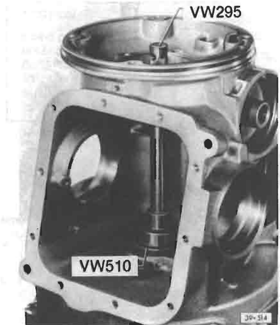
Fig. 8 Pinion bearing outer race, installing — drive in until seated
