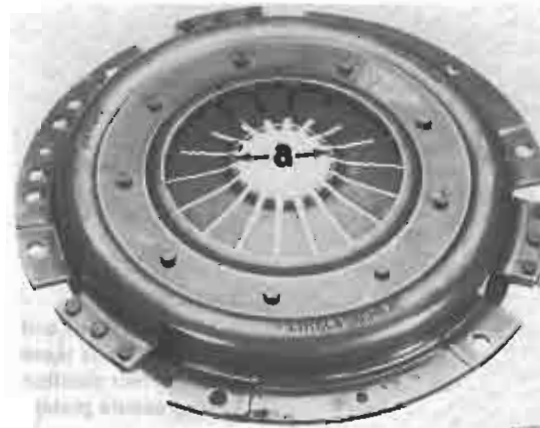
Fig. 4 Clutch pressure plate, 228 mm (9 in.) dia (modification only for air-cooled vehicles)
