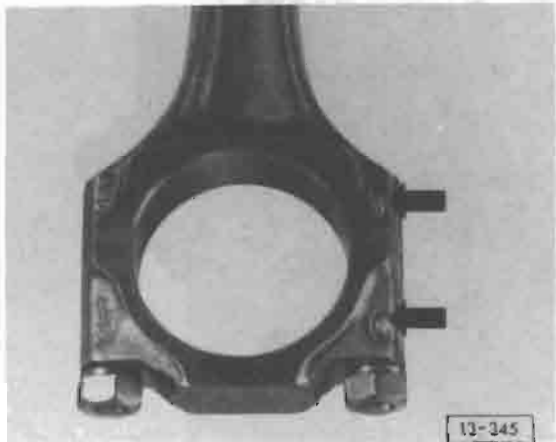
Fig. 3 Connecting rod, installing
