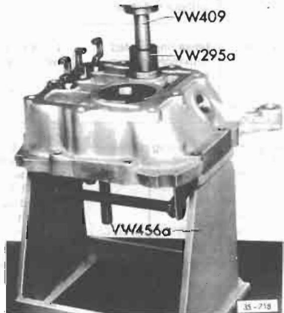
Fig. 16 Pinion needle bearing in gear carrier housing, installing
