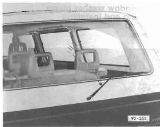
Fig. 3 Spray nozzle, adjusting — center of wiping field
