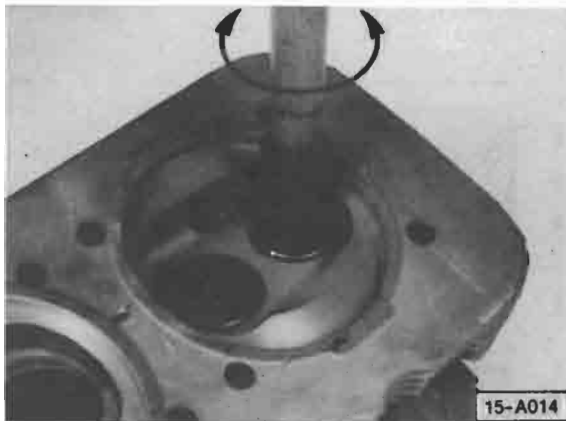
Fig. 6 Exhaust valves, lapping — lift and turn frequently
