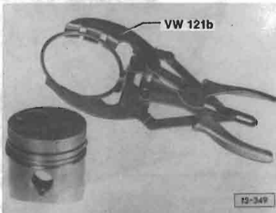
Fig. 6 Piston rings, removing/installing
