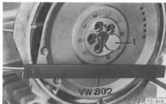
Fig. 10 Torque converter drive plate, removing
