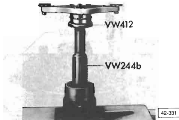
Fig. 5 Inner wheel bearing, removing
